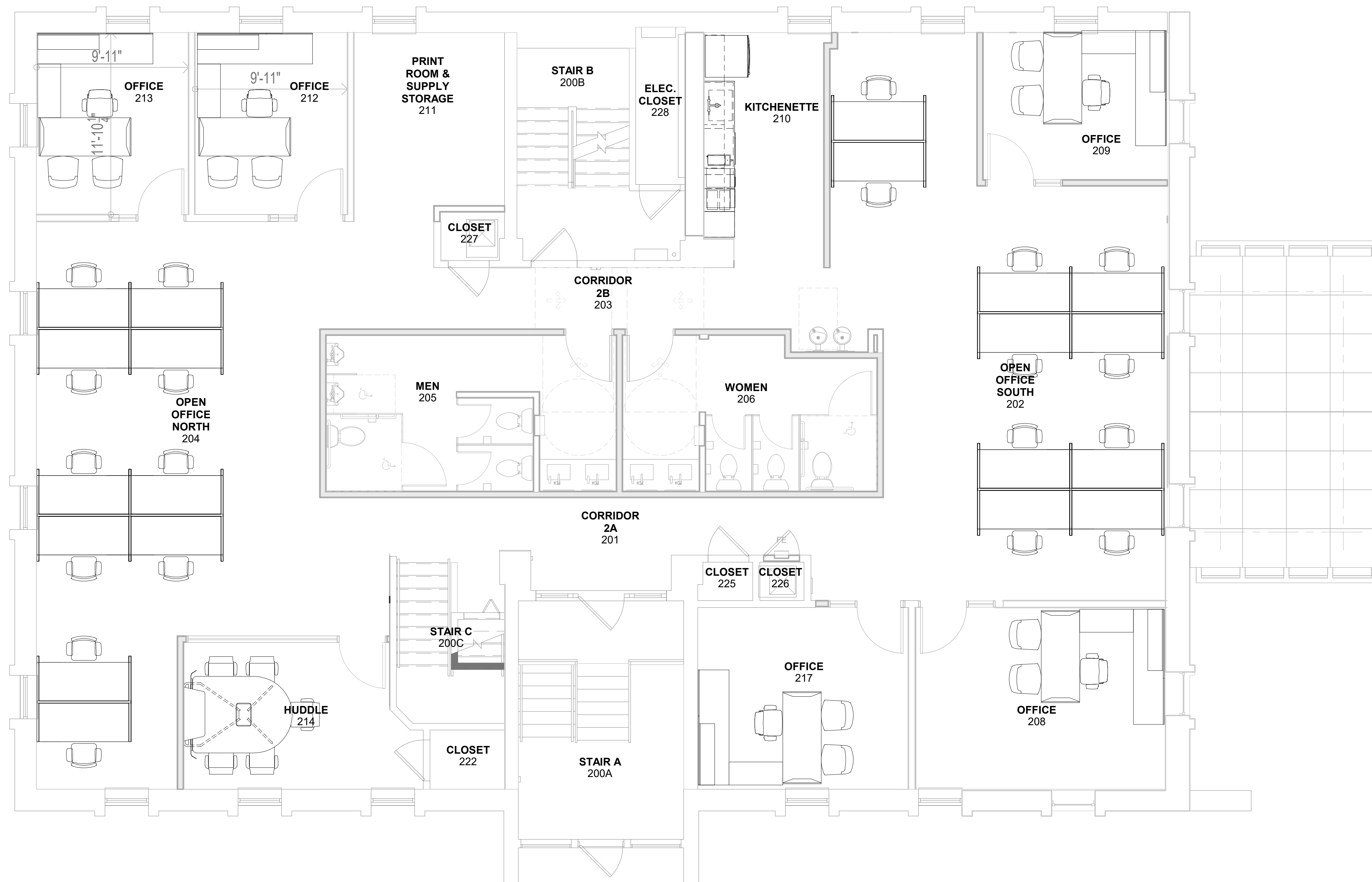
1 SECOND FLOOR FURNITURE PLAN A-142 SCALE: 1/4" = 1'-0"
